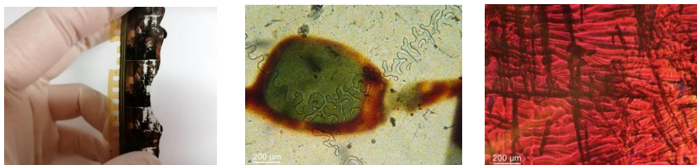
Figure 1: Optical micrographs showing the effects of the vinegar syndrome on real motion picture films made of cellulose triacetate.
